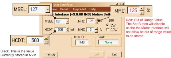
Figure 2.6.1: SPI Motor Interface Color Coding
